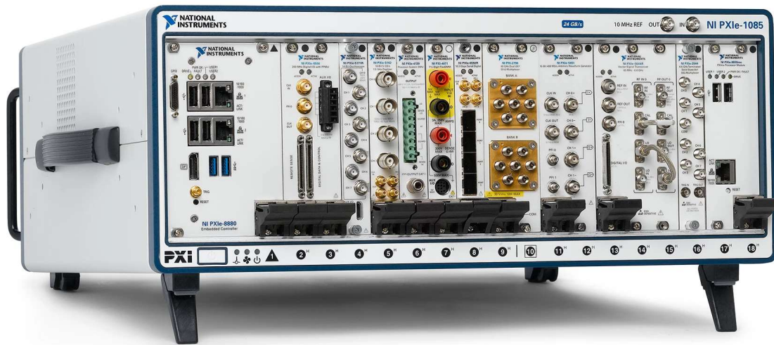
Figure 15: Illustrative figure of the NI PXIe-1085
