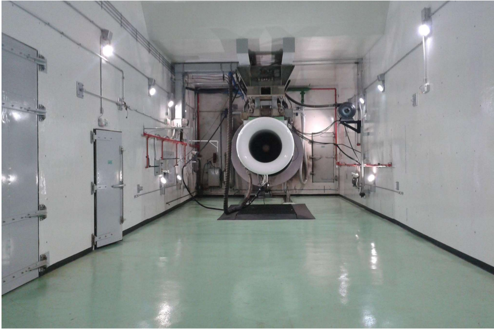
Figure 2: Inside the test cell with Spey engine installed
