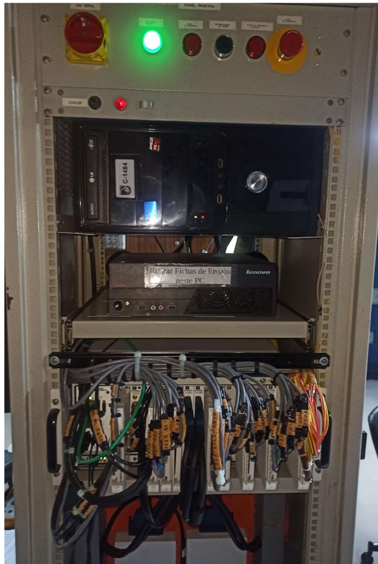
Figure 17: Figure of the GE-J85-21C and MK 807 Spey engine data acquisition system
